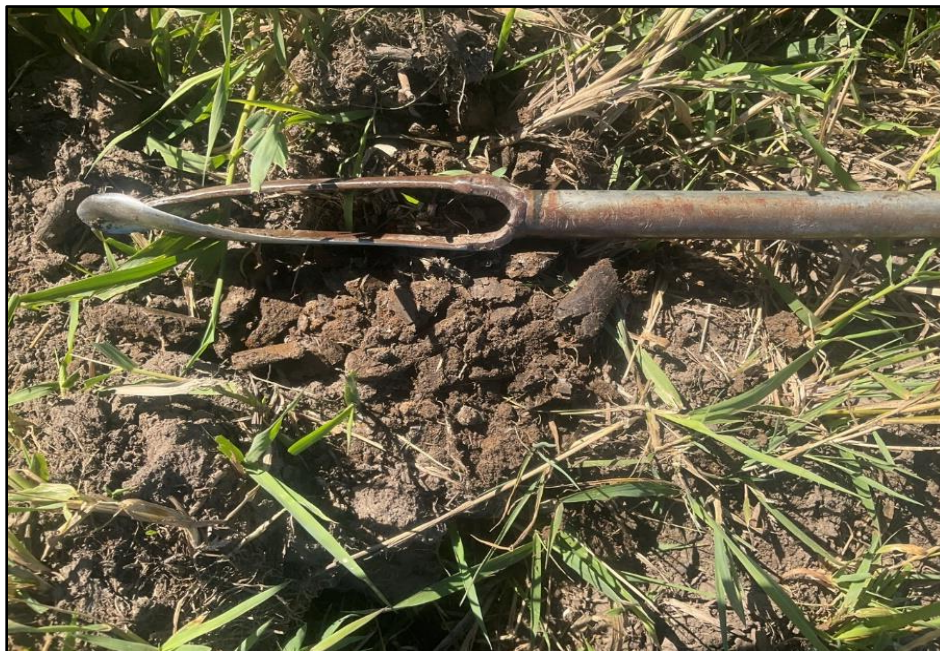
Photo C-4: Photograph of a soil test pit in W2245 consisting of silty clay and mottles at 15 cm. UTM: 12U, 434652E/5805028N (September 14, 2022)
