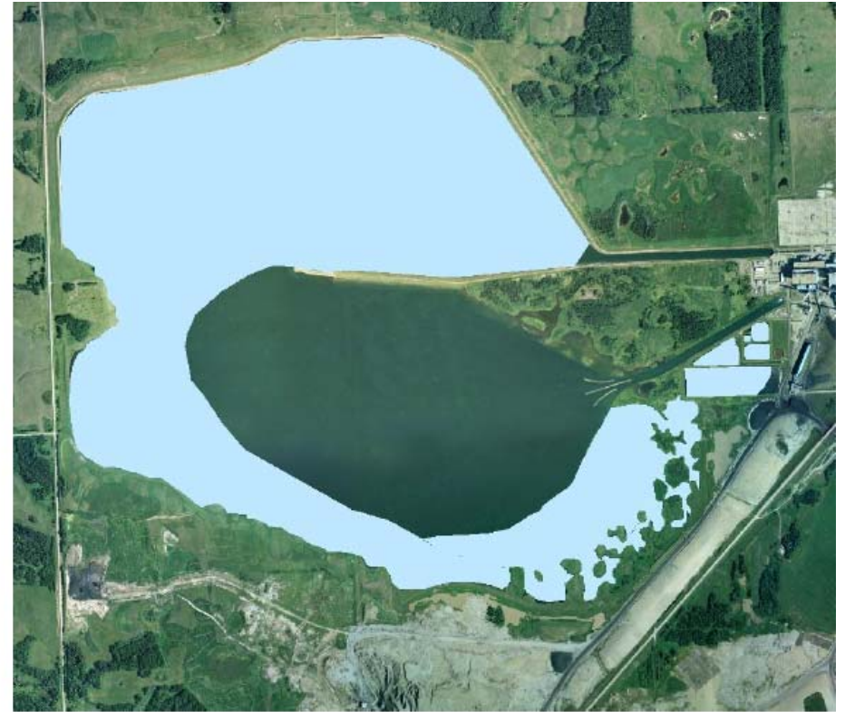
Figure A-1c: Predicted Ice Coverage and Thickness vs. Observed Ice Coverage on the Genesee Cooling Pond, December 2012.
