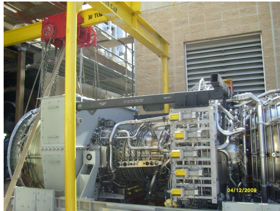
LM6000 PD ready to be installed in package
